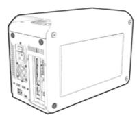
Securely close the top cover of the SAPPHIRE GearBox using the same 4 screws. Please make sure they are tightened properly. You are now ready to proceed with connecting the SAPPHIRE GearBox to your system.
