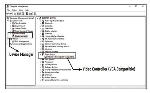
**9** To verify if the graphics card is ready to use, please go to the 「Device Manager」 to check that the graphics adapter is correctly identified and installed as shown.
