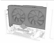
Place the graphics adapter into the SAPPHIRE GearBox and plug into the PCI-Express x16 bus. Please make sure the graphics adapter is carefully and correctly installed as shown.
