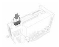
For those graphics adapters that need additional external power consumption, the SAPPHIRE GearBox offers additional connectors through the power supply. Please carefully plug the external power cables securely into the graphics adapter's power connectors as shown
