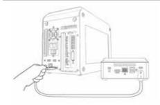
Connect the Thunderbolt™ 3 cable to both the SAPPHIRE GearBox and your device.
